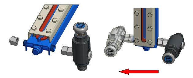
Installation weight-loaded valve, connection changed from the right side to the left side.
